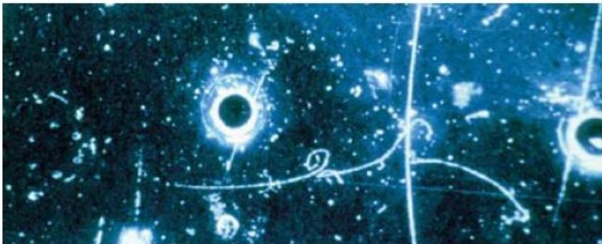
Fig. 2. The first leptonic neutral current event. An antineutrino coming from the left knocks an electron forwards, creating a characteristic shower of electron-positron pairs.
