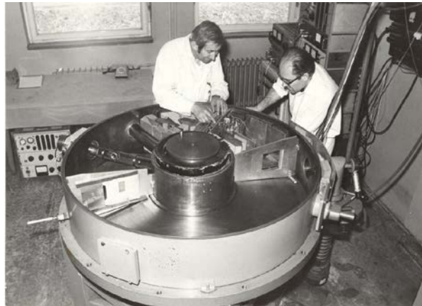
Magnetic \beta -ray spectrometer. One of the first Czech instruments operated by a computer (1971)
