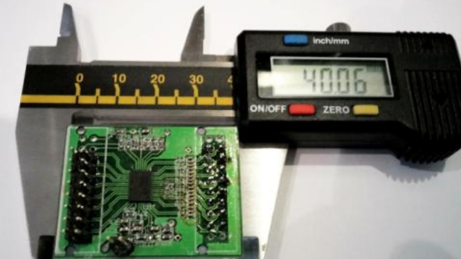
Readout Electronics developed for TPC, TOF, and ECAL (64 ch, 13-bit, 65 MSPS)
