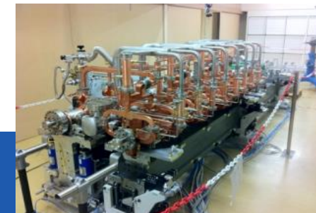
Various RF elements of a complete module, X-band test stand
