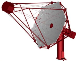
Figure 3: The baseline design for the 12 m diameter MST of Davies-Cotton type, with 8° FoV and 1500
