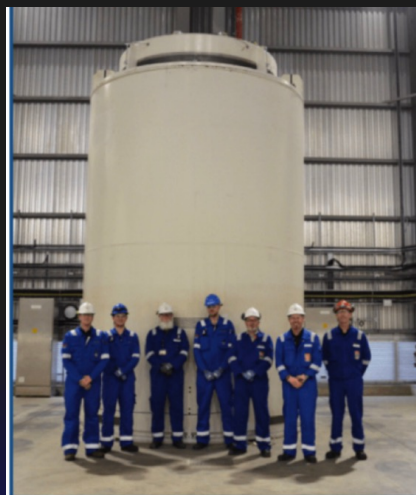
Spent fuel dry storage cask
