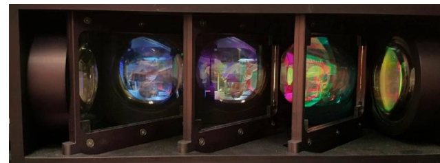
Light concentrated onto the PMTs photocathodes.
