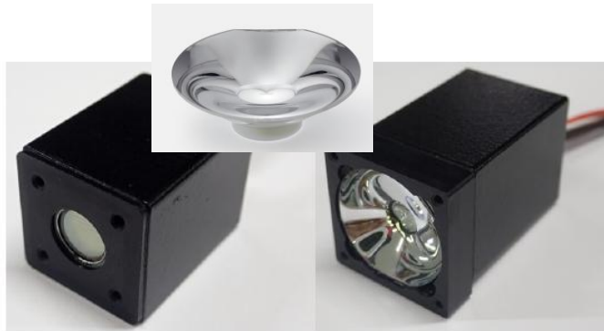
Fabricated sample of developed lens and a PMT model having it mounted on.
