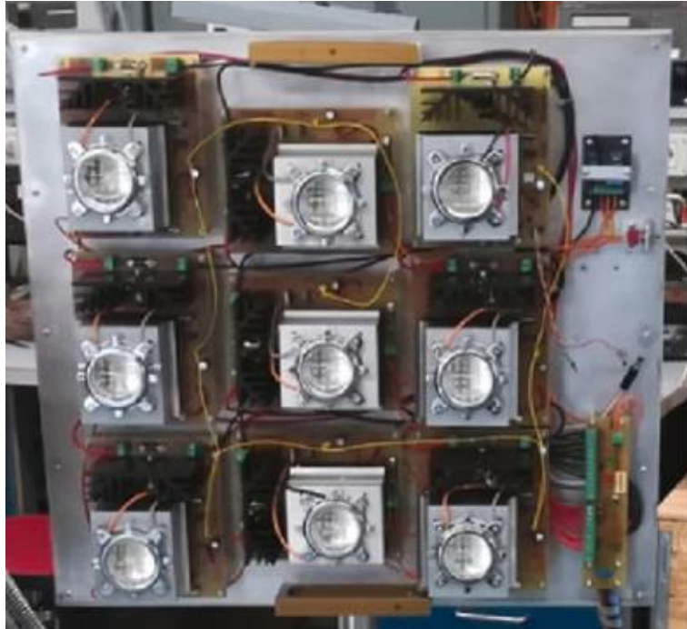
Left: array of 9 100 W COB-UV LEDs driven by an Arduino board.
